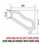
80'LIK İKİLİ GRAY GASKET (KSR 008) 80 DOUBLE WITH GRAY GASKET
